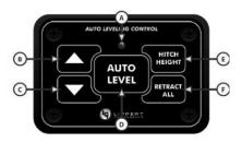
NOTE: Pressing both the arrow buttons simultaneously turns on the touchpad. Touchpad will time out after 7 minutes of non-use.
