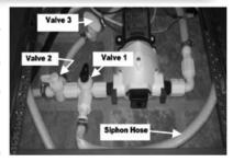
Fig. A - Water Valves (configured for Normal Operation)
